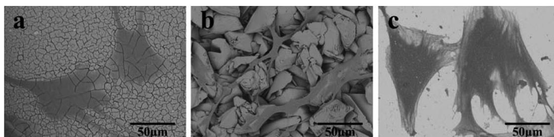
Figure 5. Morphologies of rBM-MSCs adhered on surface of JDBM (a), C-JDBM (b), and 316L (c) samples after 24 h of culture. Filopodia were tightly adhered on the substrates of the Ca-P coating (b).
